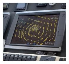
This image, and other experiences of RODA members, confirms the degradation of marine radar within wind arrays.
