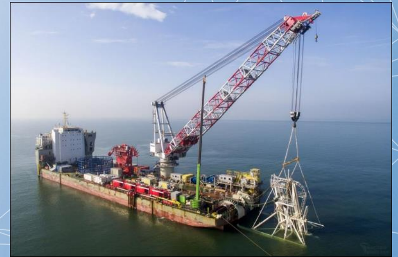
Large Towed jetting sled ~8m/25' burial depth For shallower water, has optional chain cutter for harder soils
