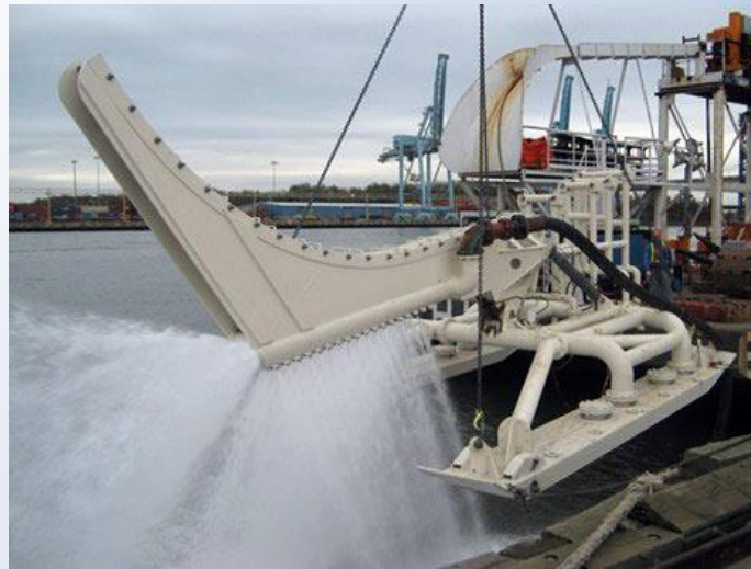
Towed jetting sled ~3m/10' burial depth For shallower water & softer soils
