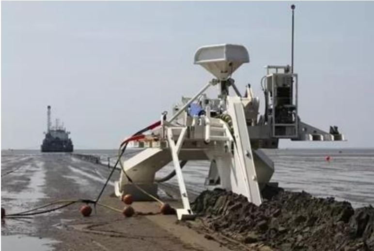
Towed Plow ~3m/10' burial depth 15m long, 6.5m wide Weighs approx. 50T
