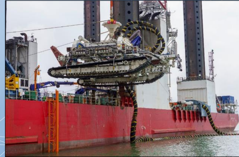
Tracked Trencher Van Oord's 'Deep Dig-It' Weighs 125T, jetting and chain cutting up to 5.0m burial depth
